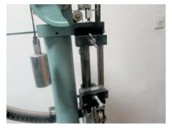
Fig. 2. Suture material placed in the Toyoseiki AT-L-L118B testing machine
